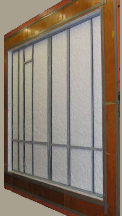
2x4 Steel Stud Wall With Local Aerogel Insulation
